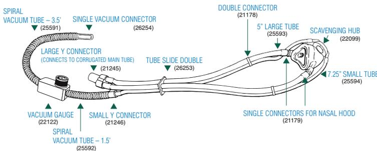
**Note:** If using RFS & Accu-Vac Scavenging Circuit, parts 25591, 22122 and 25592 are replaced with a 6' Spiral Vacuum Tube (part 26196).
