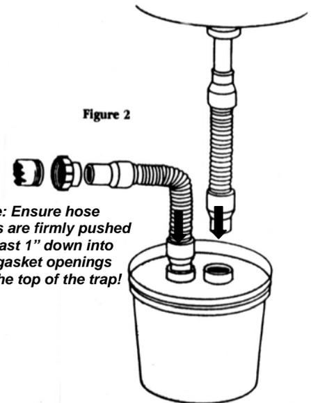
**Note: Ensure hose ends are firmly pushed at least 1" down into the gasket openings on the top of the trap!**
