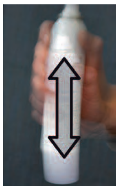
Shake the spray can again between individual bursts.
