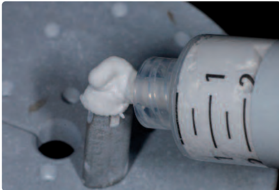
Apply IPS Object Fix Flow on the IPS e.max CAD Crystallization Pin.
