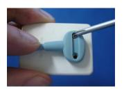
Using the screwdriver provided, loosen and remove the 2 screws that secure the cable to the Sensor. If silicone gel is present, remove this material and discard it. Dispose of the screws as new ones are supplied. Remove the cable from the Sensor.
