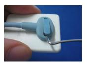
Using a dental instrument, carefully lift and remove the tab cover from the back of the Sensor cable. Dispose of the tab cover as a new one will be used when the new cable is attached.
