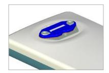
Using tweezers, remove the small elastomeric strip from the Sensor. Dispose of this strip, as it will be replaced.
