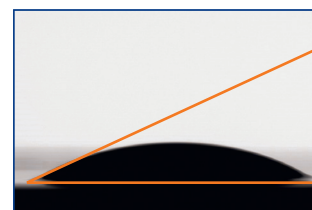
Figure 3: Impregum Garant L Duo Soft® – contact angle of ~ 24°
