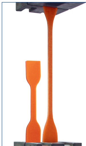
Figure 4: Stretching of V-Posil X-Light Fast
