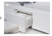
Remove the wash water tank\* and install the zirconia cooling-water tank. Then, switch the device to the wet milling mode before starting milling.
