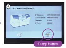
Press the Pump button on the touch panel to wash the inside of the pump.
