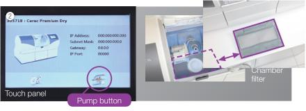
Set up the glass ceramic cooling-water tank. Press the Pump button on the touch panel to wash away any glass ceramic powder that is inside the milling chamber. Then, thoroughly flush milling debris from the milling chamber filter and milling powder from beneath the milling chamber filter.
